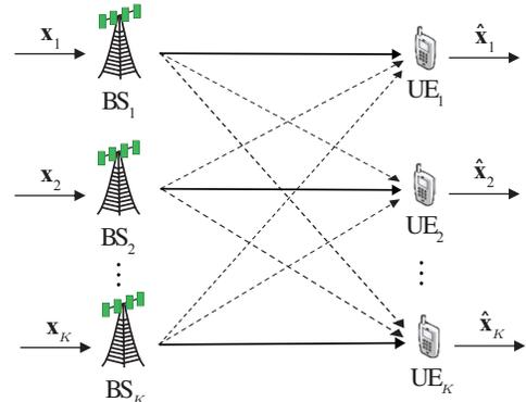
Fig. 1. The  $K$ -user MISO IC. Each base station  $BS_i$ , equipped with  $K$  antennas, has a message for each single-antenna user equipment  $UE_i$ .
