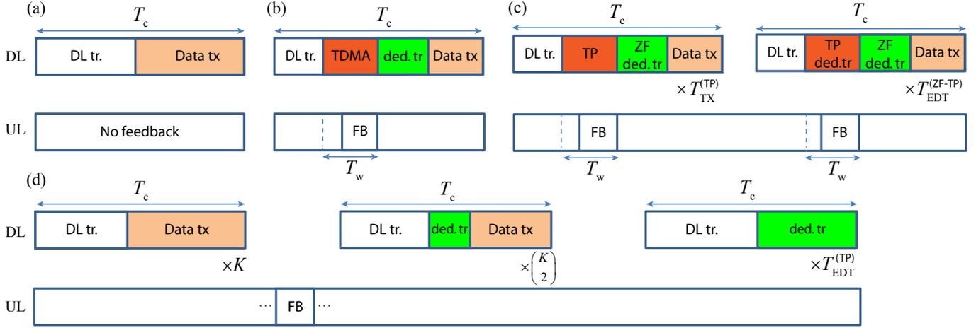
Fig. 2. Protocol frames for the downlink and uplink of (a) TDMA, (b) ZF-TDMA, (c) ZF-TP, and (d) pure TP.
