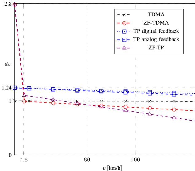
Fig. 3. Net DoF vs. UE velocity for  $\epsilon = 0.7$ ,  $K = 4$  users and  $T_w = 1680$ . Net DoF are independent of the feedback method except for the TP protocol.  $\gamma = 1$  is set since additional repetitions do not provide net DoF gains.
