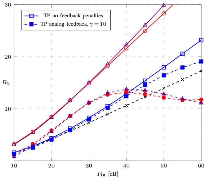
Fig. 4. Net sum-rate [bps/Hz] vs. SNR for  $v = 5$  km/h. Colors and markers identify protocols as in Fig. 3. Line styles denote different feedback settings, with  $B = 14$  bits used for digital, and  $P_{UL} = 14$  dB for analog feedback.
