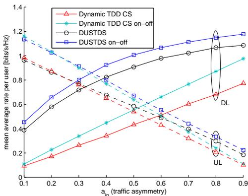
Fig. 4: Mean average per-user rate (in bits/s/Hz) in DL and UL vs.  $a_{i_n}$ .  $N = 6, I_n = 4, S = 100$ .
