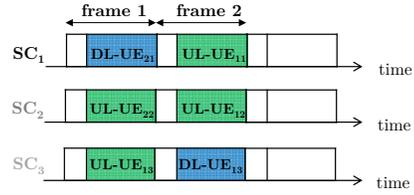
Fig. 2: Dynamic TDD in SCNs. At each frame every SC schedules one user in one transmit direction (DL or UL). An example of the user scheduling and transmit direction selection is shown for frame 1 and frame 2.
