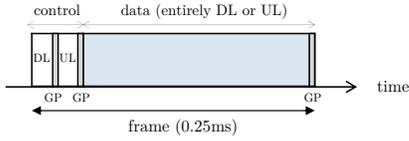
Fig. 1: Frame structure suggested for dynamic TDD [12].
