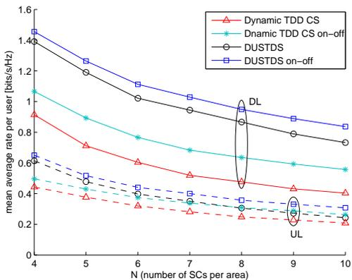
Fig. 5: Mean average per-user rate (in bits/s/Hz) in DL and UL vs.  $N$ .  $I_n = 4, S = 100, a_{i_n} = 0.7$ .
