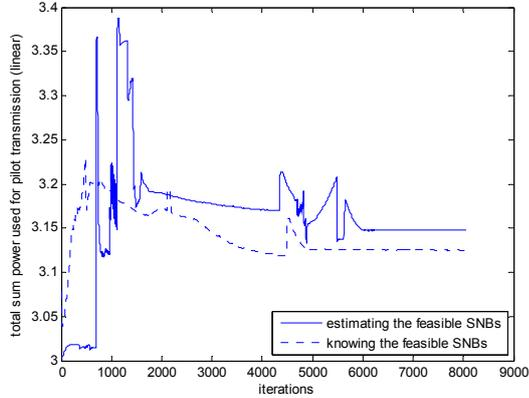
Fig. 3. Total pilot power (linear scale in W) assuming that  $\mathcal{B}_i$  is known (dotted line) or estimated (solid line).  $n_i^{listen} = 2 \quad \forall i$
