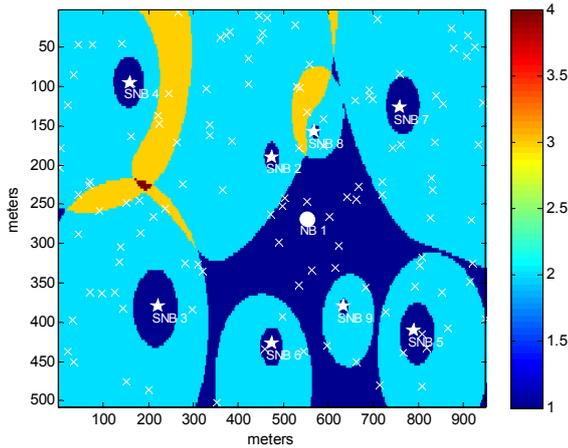
Fig. 4. Coverage area after imposing that all UEs should listen at least 2 SNBs. Color indicates the number of SNBs detected in a given location.
