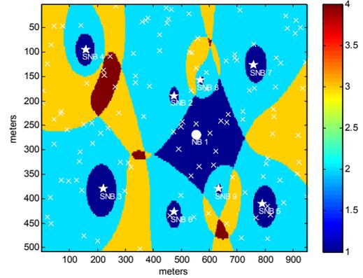
Fig. 2. Deployment of SNBs over a certain area, with 1 NB (solid circle) total  $P_{max}=40$  dBm, 6 SNBs with total  $P_{max}=24$  dBm (solid squares), 2 SNBs with total  $P_{max}=13$  dBm, and 120 UEs (crosses). Color indicates the number of SNBs detected in a location (SNBs use 30% of its  $P_{max}$  for pilot transmission).
