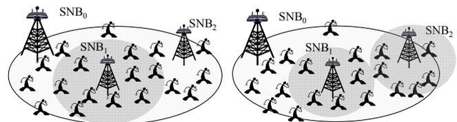
Fig. 1. Coverage area provided by Small Node B (SNB) network. Left) SNB<sub>2</sub> is switched-off, while SNB<sub>0</sub> and SNB<sub>1</sub> have 10 and 9 UEs, respectively. Right) By switching-on SNB<sub>2</sub>, the overload of the system is reduced: here SNB<sub>0</sub>, SNB<sub>1</sub>, and SNB<sub>2</sub> provide coverage to 7, 6, and 6 UEs, respectively.
