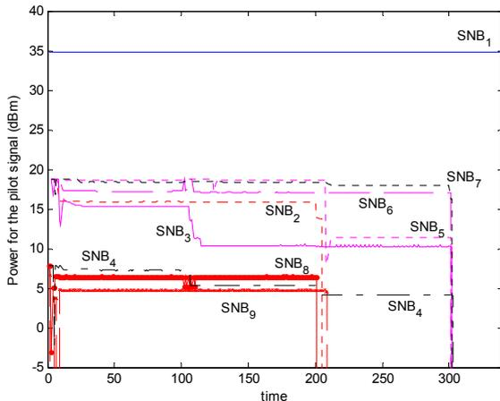
Fig. 5. Pilot power (in dBm) evolution of the different SNB when at  $t = \{0, 100, 200, 300, 400\}$  there are  $N_u = \{120, 96, 60, 24, 6\}$  active UEs.
