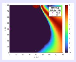
On the other hand, we have also developed a transmission strategy based on a BS endowed with a RIS composed of several elements. Each individual element of the RIS can act as a transmitting antenna or as a reflector whose reflection characteristics can be changed by the BS in real-time during the transmission depending on the symbols to be transmitted.
