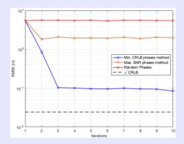
This outperformance has proven to be robust to the variation of some key system parameters (RIS size and transmission SNR). In addition, we have achieved positioning accuracy values comparable to the theoretical CRLB.
