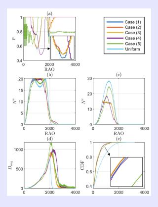
Figure shows some KPIs (optimized ACB parameter p in a), Number of served MTCDs  $N_s$  in b), Number of collisions  $N_c$  in c and average delay  $D_{avg}(d,e)$  of the served MTCDs in terms of time. Results have been averaged over 1000 simulation runs.
