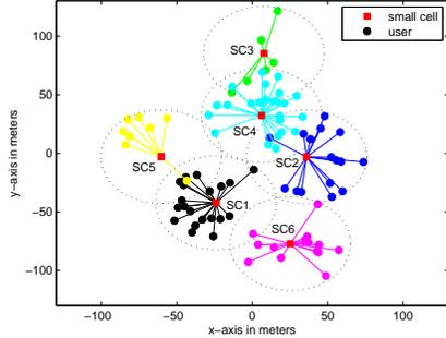
Fig. 3: Example of network deployment used for simulations with  $K = 6$  SCs. The number of users at each SC is: 20, 16, 6, 24, 8, 15, respectively.
