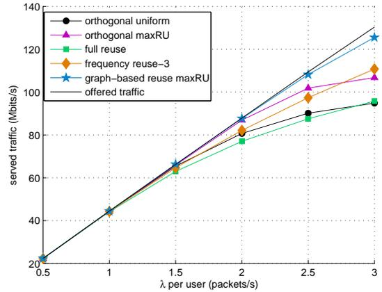
Fig. 6: Served traffic (in Mbits/s) versus packet arrival rate per user ( $\lambda$ , in packets/s).
