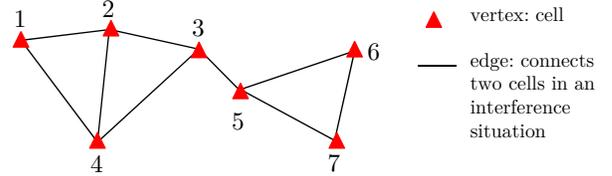
Fig. 1: Interference graph for a network of  $K=7$  cells.
