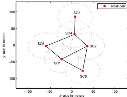
Fig. 4: Interference graph associated to the network deployment in Fig. 3. The threshold distance is 80 m.
