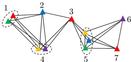
Fig. 2: Extended graph of the interference graph in Fig. 1.  $K=7$  cells,  $N=5$  resources,  $x_1^* = 2$ ,  $x_2^* = 1$ ,  $x_3^* = 1$ ,  $x_4^* = 2$ ,  $x_5^* = 3$ ,  $x_6^* = 1$ ,  $x_7^* = 1$ .
