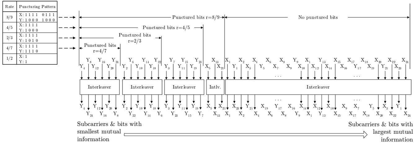
Fig. 1. RCPC based interleaver pattern. Example for IEEE802.11a.  $K=48$ ,  $N=2$ ,  $P=8$ ,  $b=1$  (BPSK constellation).
