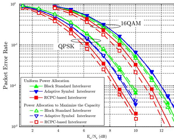
Fig. 3. PER comparison for different interleavers. Power allocation strategy: uniform (solid lines) and max. capacity (dotted lines).
