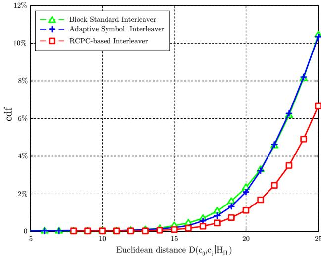
Fig. 2. Cumulative density function of the squared Euclidean distance for different interleavers.
